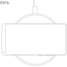
3. Keep your phone centered on the Mi Wireless Charging Pad while charging. Adjust the position of your phone if it is not charging, the green LED light should come on and your phone's status should change to "Charging" (Please refer to figure below for placement).
