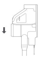
Pull the vacuum down in the docking station to charge
