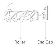
4. After cleaning, install the end cap back on the roller.
