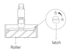
2. Turn the end cap to the open position. Gently slide the roller away from the head.
