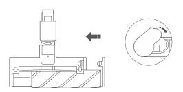
6. Rotate the latch clockwise by 90° to the locked position to secure the roller.
