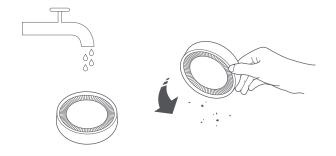
4. To thoroughly dry the filter, keep it in a ventilated or cool place for at least 24 hours after cleaning.
