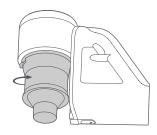
4. Slightly tilt the dust compartment when installing it on the vacuum.
