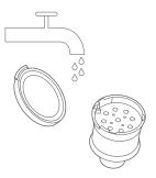
5. To thoroughly dry the filter and cyclone assembly, keep them in a ventilated or cool place for at least 24 hours after cleaning.
