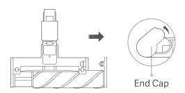
3. Separate the end cap from the roller and remove any hair wrapped around the roller and end cap.
