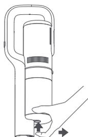
The dust cup disassembling: turnover the dust cup, remove the filter, pull the handle upward in the same direction and take out the cyclone mechanism
