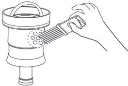
2. The dust cup and metal mesh cleaning: clean the dust cup and metal mesh with clean water and use after drying to prevent dust caking.
