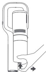
Dust Dumping: dump the uncovered cup on garbage collection device for dumping.
