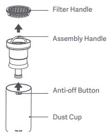
Install uncovered dust cup: click the anti-off button, insert the dust cup following the diagram counterclockwise until you hear it clicks
