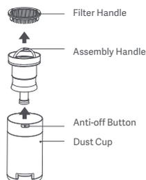
Dust Dumping: dump the dust cup with cover on garbage collection device for dumping.
